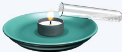
Image 9. The carbon dioxide suffocates the candle's flame.
