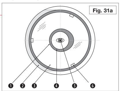
Fig. 31a is showing the view through a correctly collimated Newtonian telescope as seen through a focuser without eyepiece.
