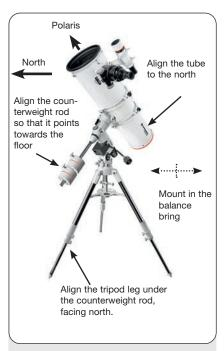
Fig. 16a: The parallactic home position, side view
