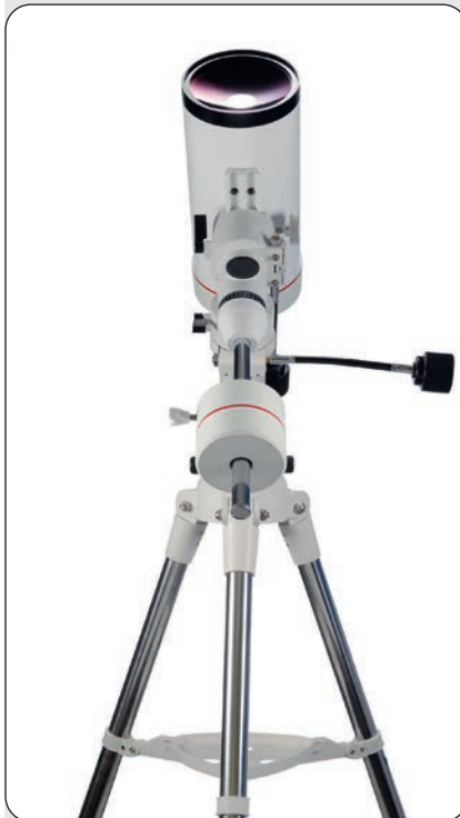
Fig. 4 The parallactic home position seen from the North.
