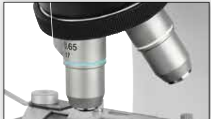
Semiplane Objektive (inkl. 100x Öl) Semi-plan objectives (incl. 100x oil)
