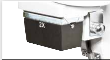
Wechselbare Objektive Changeable objectives
