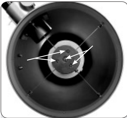
Fig 31b: The four collimation screws on the secondary mirror housing
